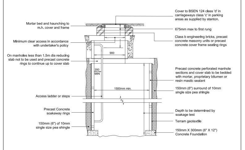
Pipework joint to be as close as possible to face of manhole to permit satisfactory joint and subsequent movement
