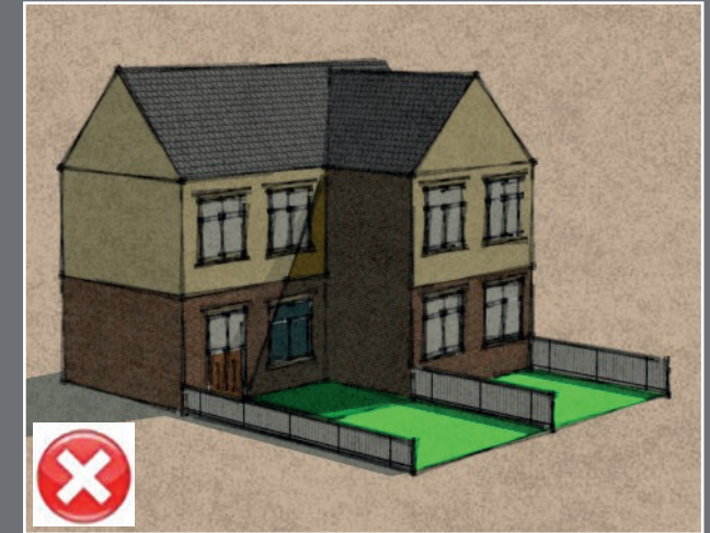
Figure 10.3: An oversized two storey rear extension that results in a loss of light and has an overbearing impact on the adjoining property
