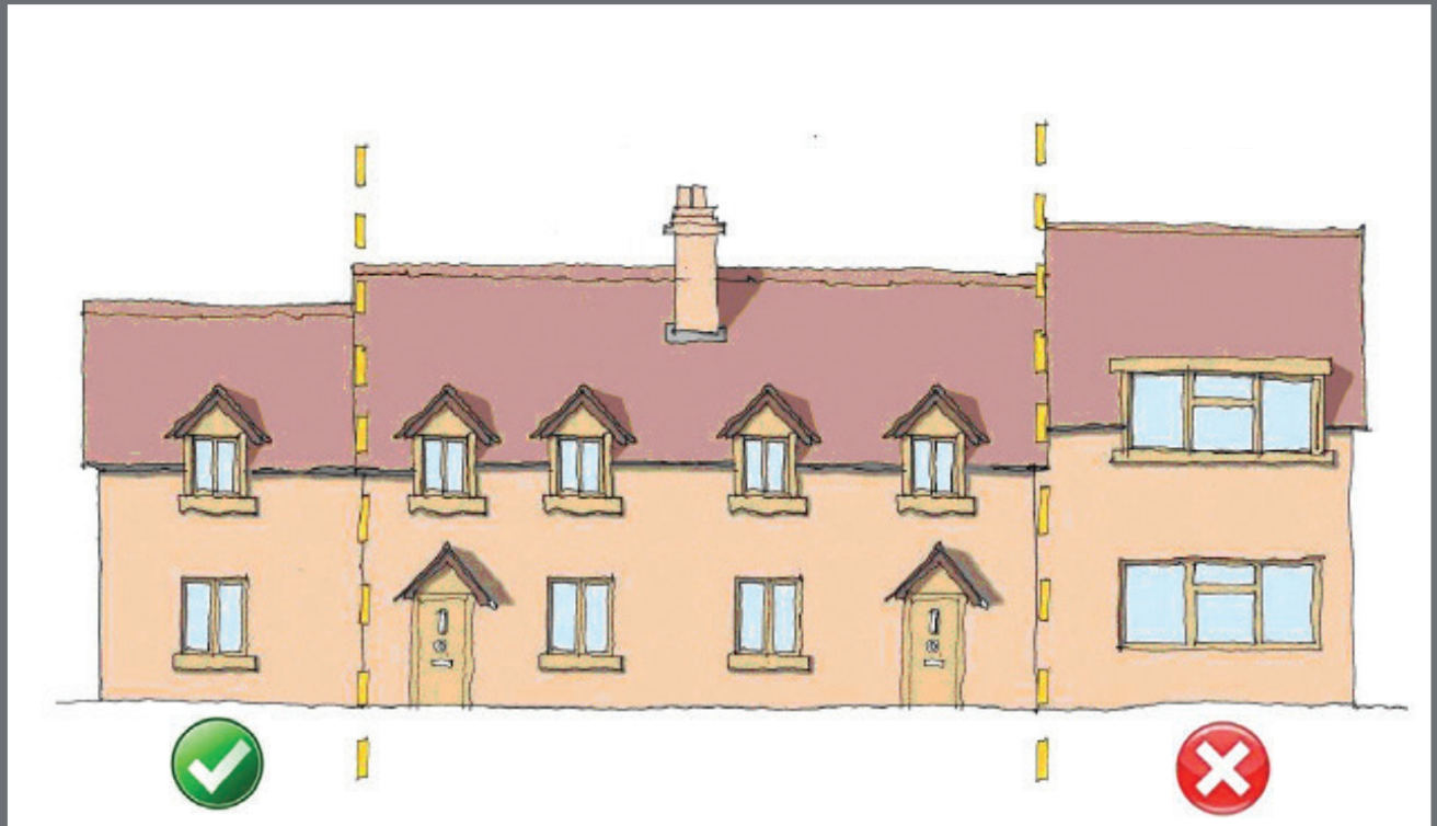
Figure 10.1: Acceptable and unacceptable side extension designs
