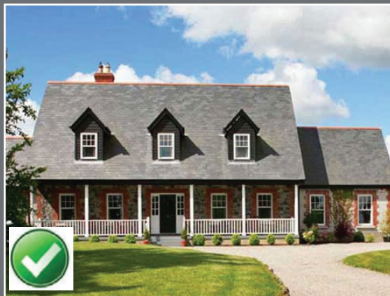
Symmetrical glazing that is well proportioned and taller on the ground floor than at upper levels
