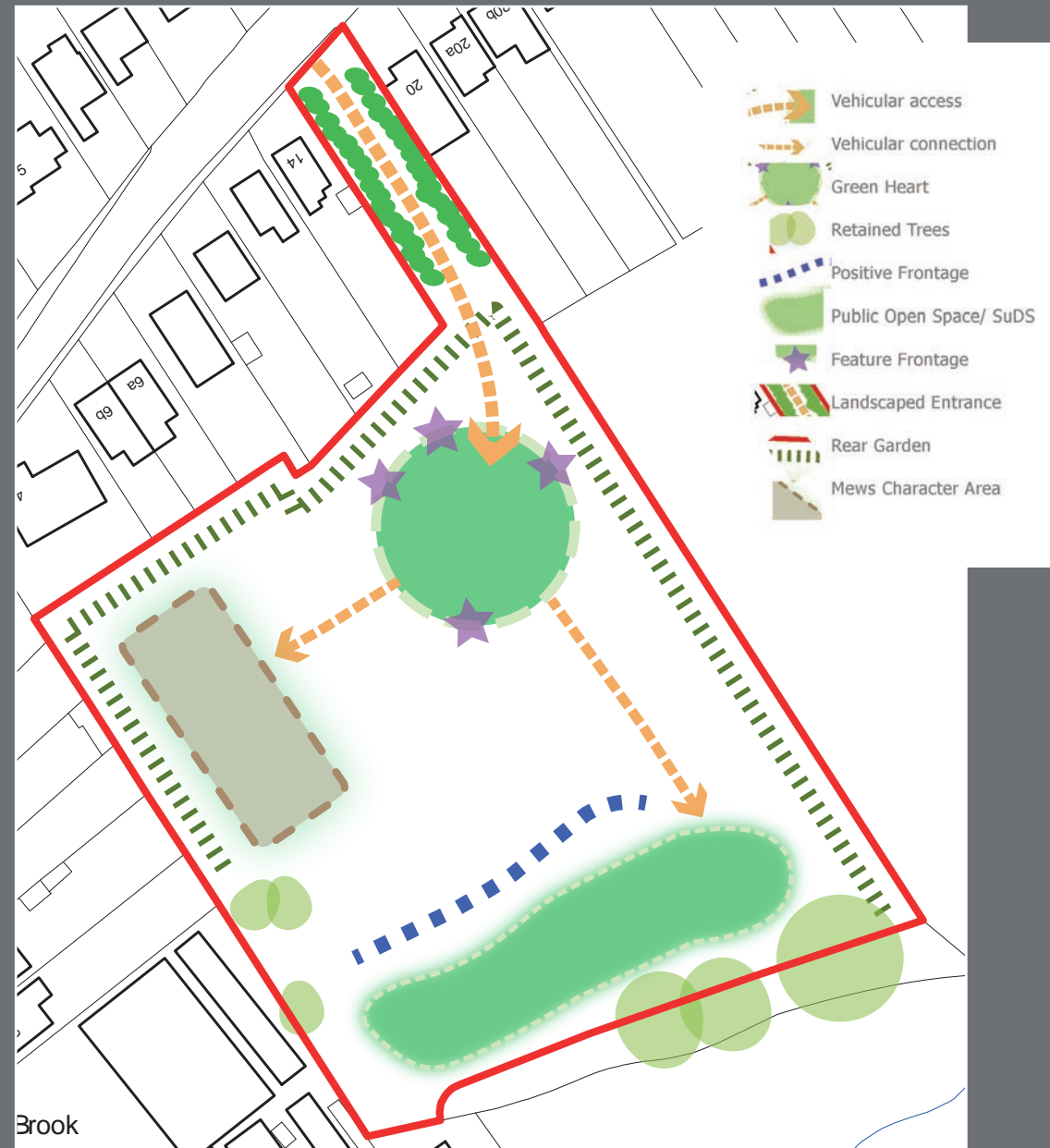
Figure 5.1: Illustration of a Concept Plan Example reproduced with permission of Thakeham Homes & Barton Willmore
