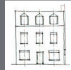
Figure 10.4: Dormer windows need to complement and align with the fenestration of the façade
