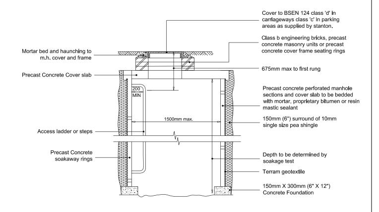
Pipework joint to be as close as possible to face of manhole to permit satisfactory joint and subsequent movement
