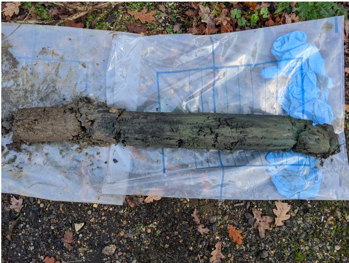
Photograph 8 – Window sample run between 2.0m and 3.0m bgl within WS106.
