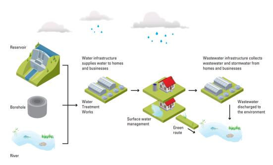
A broad overview of the interaction between the water environment and water and wastewater infrastructure is illustrated in Figure 4-1. Wastewater is generally produced following the use of potable water in homes, businesses, industrial processes and in certain areas can include surface water runoff.
