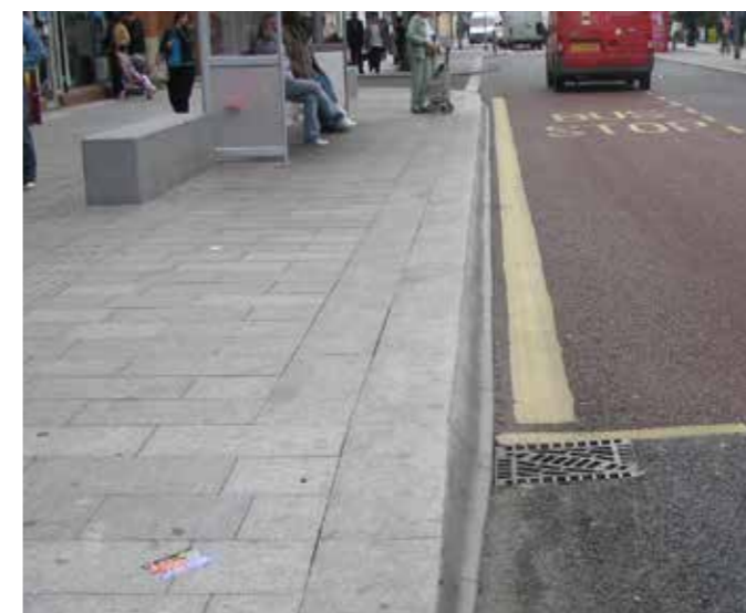
Locally raised bus stops allow for easy access and integrate seating and bus shelters.
