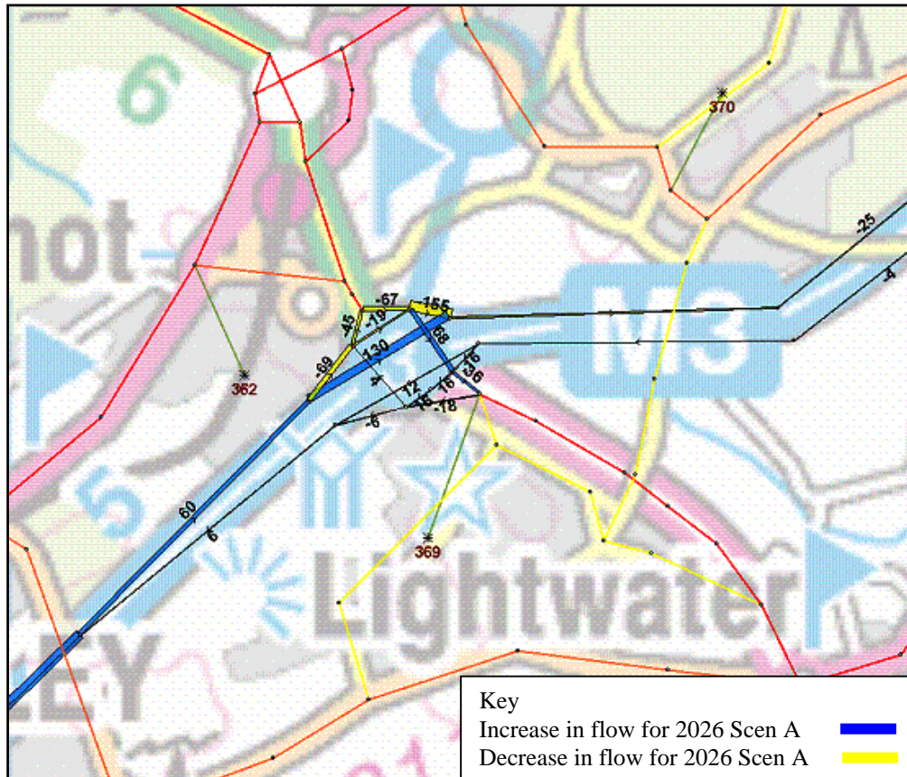
Figure 5.40: 2026 Scenario A flow minus the 2026 Do-Minimum flow (results in the increases/decreases in flow between the 2026 Do-Minimum and 2026 Scenario A being displayed).
